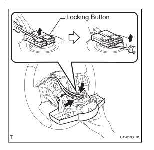
(b) Pull the steering pad out of the steering wheel assembly and support the steering pad with one hand as shown in the illustration.
